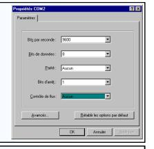
The PC is now in terminal mode, connect it to the device by plugging the RS232 cable. The measure is now displayed on the terminal. To access configuration, press 'C' key.
